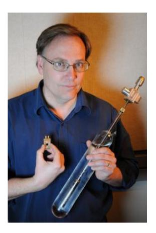
NIST physicist Samuel Benz holds the two components that are compared in the first electronic measurement of the Boltzmann constant. The ac reference signal generated by the superconducting chip (left) is compared to the "Johnson noise" of a resistor inside the glass container (right). In the experiment, the water in the container is held at its triple point temperature near  $0^{\circ}$  C or  $32^{\circ}$  F. Credit: Burrus/NIST
