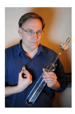
NIST physicist Samuel Benz holds the two components that are compared in the first electronic measurement of the Boltzmann constant. The ac reference signal generated by the superconducting chip (left) is compared to the "Johnson noise" of a resistor inside the glass container (right). In the experiment, the water in the container is held at its triple point temperature near 0° C or 32° F. Credit: Burrus/NIST
