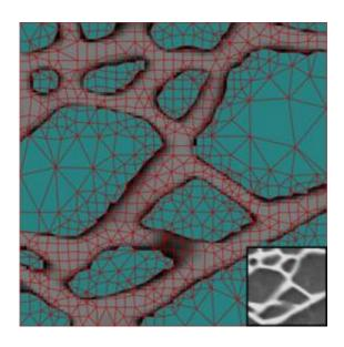
Once provided with a microscope's image of a composite material (inset), OOF software can help analyze the effects of the material's internal structure on stress. Using OOF, researchers can identify the different substances (blue and gray areas) that make up the material and compute their response to stress or other effects, providing clues about how the overall sample will behave. Credit: Langer, NIST
