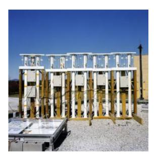
Mounted on the roof of a building on NIST's Gaithersburg, Md., campus, this NIST-developed device is designed to induce temperature-caused strains on sealant specimens while monitoring loads and displacements. Affixed to a rigid base, the top segments of PVC pipe expand and contract with changes in temperature. Sensors, load cells, and specimens--sandwiched between aluminum blocks--are suspended from the top crosspiece, which moves, and are attached to the same rigid base. Credit: NIST
