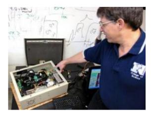
Physics professor Pat Arnott of the University of Nevada, Reno explains the new technology for photoacoustic air particle monitoring recently licensed by the University to Droplet Measurement Technologies. The device is used to measure air quality, including black carbon, in a number of applications. Credit: Photo by Mike Wolterbeek, University of Nevada, Reno.
