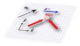
The researchers create a synthetic electric field (E\*) in an ultracold gas of several hundred thousand rubidium atoms (BEC) immersed in a constant magnetic field (B0). Using lasers (red arrows), the team alters the atoms' energy-momentum relationship, which causes the atoms to move in a way that is physically identical-and mathematically equivalent-to how a charged particle would move in an electric field. Credit: NIST
