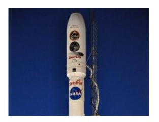
The Orbital Sciences Taurus the XL rocket and NASA's encapsulated Glory spacecraft awaiting an early morning launch on the pad at Space Launch Complex 576-E at Vandenberg Air Force Base in California, February 2011. The earth observation satellite Glory failed to reach orbit after its protective cover did not detach following its launch.
