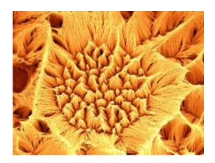
Taylor and Schroers engineered nanowires out of a novel material called bulk metallic glass in order to make fuel cell catalyst systems more durable and efficient. Credit: Golden Kumar and Miriam Schroers/Yale University
