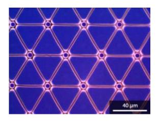
Optical microscopy image of a fully connected hexagonal network of microwires prepared by the self-assembly of gold nanoparticles on a photoresist template.
