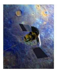
The MESSENGER spacecraft will orbit Mercury in an effort to study the geologic history, the enigmatic magnetic field, the surface composition and other mysteries of the planet. The shield visible on the probe's right side protects its sensitive instruments from the sun's intense heat. (Credit: NASA/JHUAPL/CIW)
