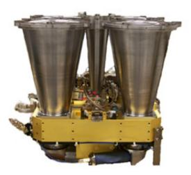
MLA maps Mercury's landforms and other surface characteristics using an infrared laser transmitter and a receiver that measures the round-trip time of individual laser pulses. Credit: JHUAPL
