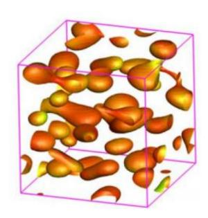
Nano-sized particles embedded in alloys can make alloys highly elastic and enable them to convert electrical and magnetic energy into movement. Credit: Physical Review Letters
