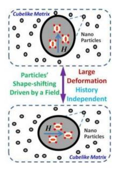
The crystal structure of nanoparticles embedded in an alloy can be realigned under an electric or magnetic field, which in-turn deforms the material. Rutgers researchers expect these alloys to show larger shape changes and output forces than traditional materials. Credit: Weifeng Rao
