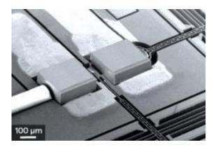
A scanning electron microscopy image of the master and slave lasers integrated onto a silicon substrate to form a miniature tunable laser. Credit: 2010 IOP
