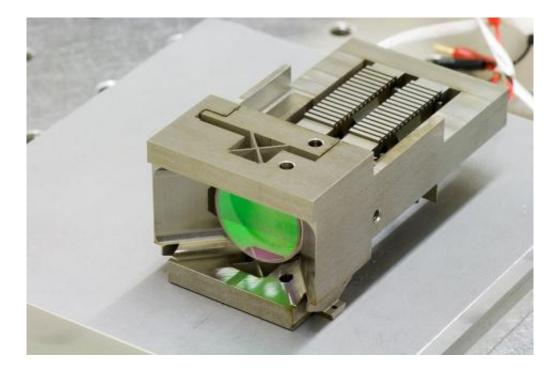
TNO-developed Point Ahead Angle Mechanism prototype for the LISA mission's laser. Credits: TNO
