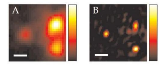
Experimental imaging demonstration with a GaP HIRES-lens. (A) A reference image taken with conventional oil immersion microscope. The image shows a blurred collection of gold nanoparticles. The scale bar represents 300 nm. (B) A high resolution image acquired with the GaP HIRES-lens. Image credit: E.G. van Putten, arxiv.org/abs/1103.3643v1
