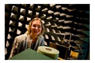
Elena Semouchkina tests a microwave dielectric cloak in an anechoic chamber--a cave-like compartment lined with charcoal-gray foam cones to abosrb sound. Credit: Elena Semouchkina, ECE Department, Michigan Tech University
