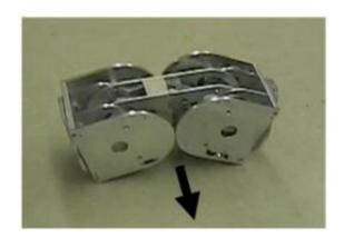
The iMobot can drive on its wheels, crawl like an inchworm, or stand up and rotate as a platform. Credit: Graham Ryland/Harry Cheng, UC Davis
