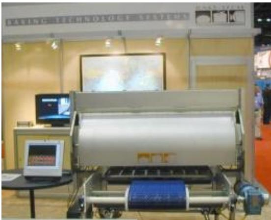
The Georgia Tech Research Institute (GTRI) has developed a production-line system that automatically inspects the quality of sandwich buns exiting the oven and adjusts oven temperatures if it detects unacceptable buns. Credit: Georgia Tech Research Institute
