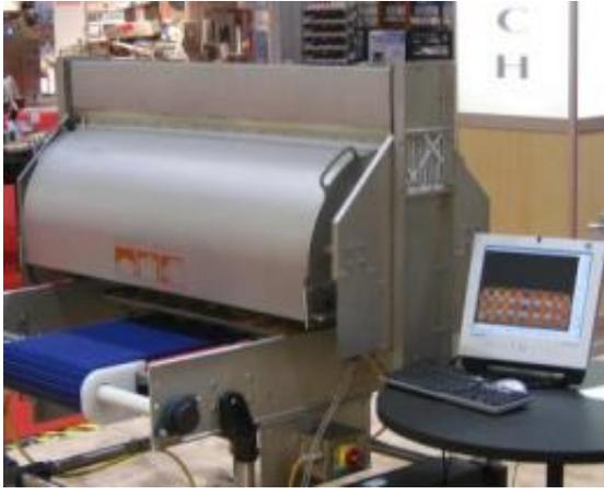
GTRI worked with Georgia companies Flowers Foods and Baking Technology Systems (BakeTech) to design a prototype imaging system to inspect the quality of sandwich buns. It has been in full-operational mode in a baking facility for more than a year. Credit: Georgia Tech Research Institute
