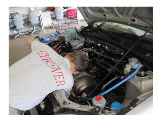
Now let's go under the hood. The standard powertrain of the Civic is replaced by a 35-horsepower electric motor that will be powered by 33 lithium-iron-phosphate batteries. The batteries take about 10 hours to charge, and they will give drivers more than 40 miles of mixed condition driving, in city and on highways, with top speeds at more than 70 miles an hour. No specific number on the top speed.
