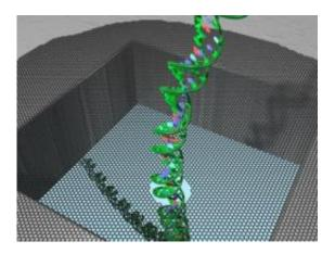
A nanopore is created in graphene to form a trans-electrode, measuring variations in current as a single DNA molecule passes through the pore. Credit: iemedia solutions/ONT
