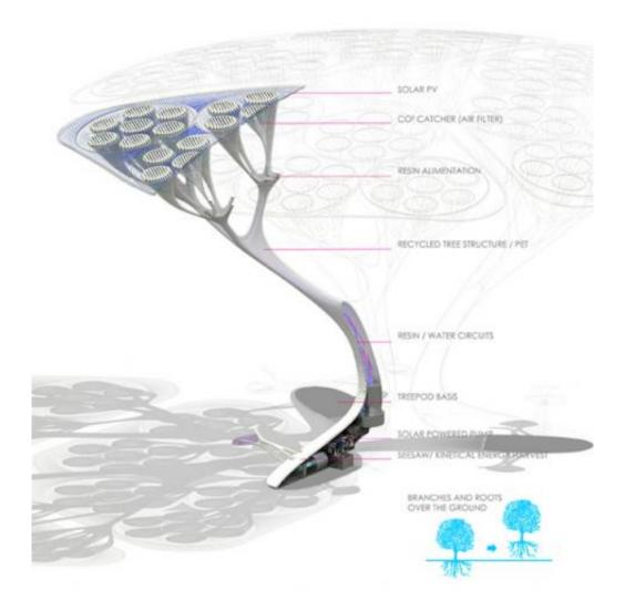
After a period of trial and error it was determined that the tress could not be powered by the sun alone. Instead of relying on plugs or batteries the secondary source of power will be the kinetic energy of humans. The groves of tree pods will be pared with hammocks and see-saws that will help to power the devices.
