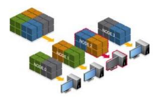
The redundant data distribution of an array showing that a node failure will leave at least one copy of the data available for continued execution. This is the basic idea that enables the approach, which can be used in many science domains.
