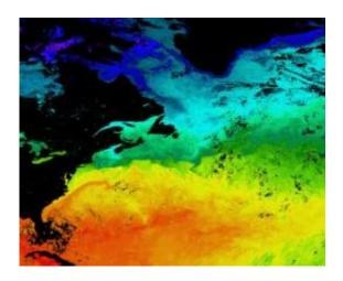
This map shows sea-surface temperatures averaged over eight days in September 2001, as measured by NASA's Terra satellite. Dark red represents warm water (32 degrees Celsius) and purple is cold (-2 degrees Celsius). The Gulf Stream can be seen as the orange strip extending from the eastern U.S. toward the Atlantic. Credit: Ronald Vogel, SAIC for NASA GSFC
