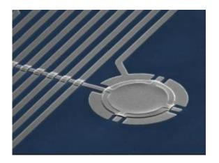
This is a colorized micrograph of NIST's aluminum drum, which is 15 micrometers in diameter and 100 nanometers thick. The drum is used in quantum information experiments and ultraprecise measurements of mechanical motion. Credit: A. Sanders/NIST
