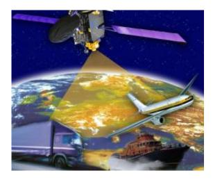
The US GPS global satellite navigation system has an accuracy of 5-10 m. Across our continent that accuracy is greatly sharpened to 1-2 m through the European Geostationary Navigation Overlay Service (EGNOS), an operational
