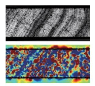
A slice of ferromanganese crust from the Pacific Ocean was analyzed using the MIT team's SQUID microscope. The top image shows a portion of the image of the slice taken with an electron microprobe. The second image shows the magnetized regions in the slice, with red areas showing one direction of magnetization and blue the opposite direction. Images courtesy of Ben Weiss
