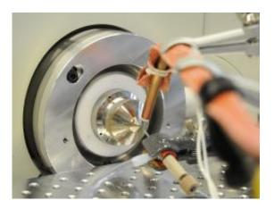
The cone (center of image) aspirates the ionised breath and feeds it into the mass spectrometer. Credit: Peter Rüegg/ETH Zurich
