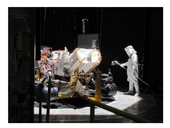
This image shows preparation for one phase of testing of the Mars Science Laboratory rover, Curiosity. The testing during March 2011 in a 25-footdiameter (7.6-meter-diameter) space-simulation chamber was designed to put the rover through operational sequences in environmental conditions similar to what it will experience on the surface of Mars. Credit: NASA/JPL-Caltech
