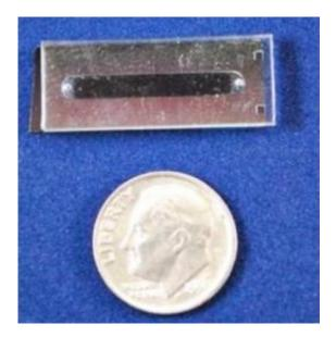
This tiny microfluidic device can separate cancer cells from normal blood cells. Image: Brian Wardle
