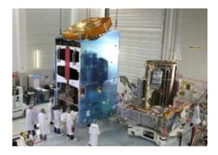
Alphabus service module and Alphasat repeater module stand side by side before the mating procedure which took place at Astrium facilities in Toulouse, France on 15 March. Credits: ESA
