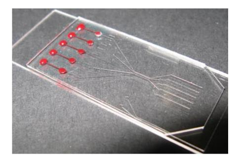
Photograph of the stand alone 1x2 inch SIMBAS chip simultaneously processing five separate whole-blood samples by separating the plasma from the blood cells
