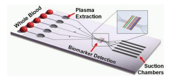
Schematic of the tether-free SIMBAS chip that shows some of the functional elements, such as the blood loading area, the plasma separation microtrenches, detection sites and the suction flow structures. Credit: Ivan Dimov
