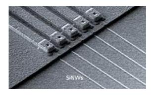
Scanning electron microscopy image of a sensor formed from five individual SiNWs. Credit: 2011 Elsevier
