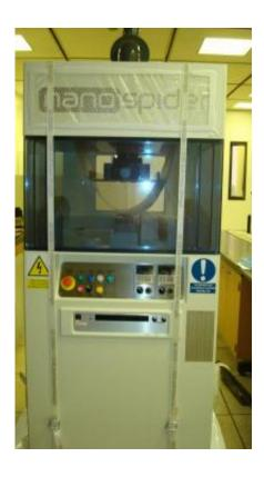
This nanospider machine is used to spin the fibers that deliver antibiotics to disable disease-producing bacteria and fungi. Credit: Elmarco s.r.o.
