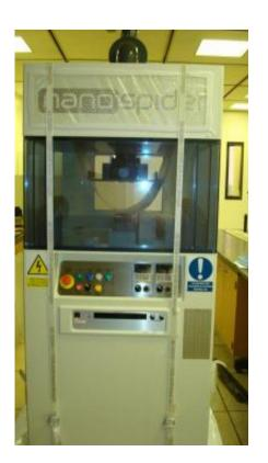
This nanospider machine is used to spin the fibers that deliver antibiotics to disable disease-producing bacteria and fungi. Credit: Elmarco s.r.o.
