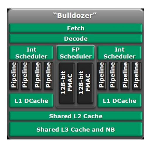
Based on the diagram AMD intends to dramatically improve multithreading performance of its CPUs: two INT schedulers, an FP scheduler and separate data caches for each of four cores. Credit: AMD
