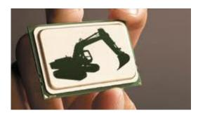
AMD's Bulldozer is a multi-threaded high performance x86 CPU that includes the 32-nm Zambezi chips with 4, 6, or 8 cores.
