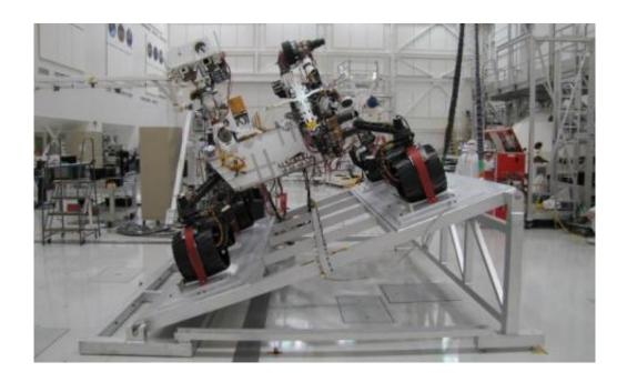
The image shows Curiosity on a tilt table in the Spacecraft Assembly Facility at NASA's Jet Propulsion Laboratory, Pasadena, California. Credit: NASA/JPL-Caltech
