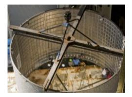
A massive 27.5-foot-diameter and 20-foot-tall fully-instrumented test article was moved into location in Marshall's Engineering Test Laboratory in Building 4619 in preparation for next month's Shell Buckling Knockdown Factor test. The polka dot pattern applied to the barrel allows the engineering team to capture precise measurements of the deformations of the test article during the test using
