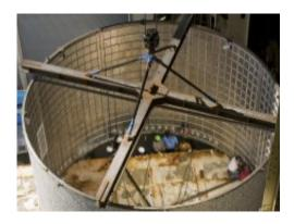
A massive 27.5-foot-diameter and 20-foot-tall fully-instrumented test article was moved into location in Marshall's Engineering Test Laboratory in Building 4619 in preparation for next month's Shell Buckling Knockdown Factor test. The polka dot pattern applied to the barrel allows the engineering team to capture precise measurements of the deformations of the test article during the test using
