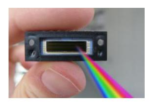
CMOS image sensors can now be covered with a transparent protective coating that is permeable to light in the UV and blue spectral range. Credit: Fraunhofer IMS
