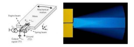
(Left) This illustration shows the entire heat engine and its electrical connections. (Right) A modified electron-microscope image shows the heat engine in motion. The amplitude of the motion in the figure is exaggerated. Image credit: P. G. Steeneken, et al. ©2011 Macmillan Publishers Limited.
