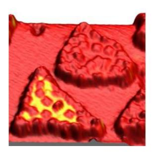
This is a scanning tunneling microscopy (50 x 50 nm2) of organic molecules. Coloring indicates variable spin orientation. Credit: CFN
