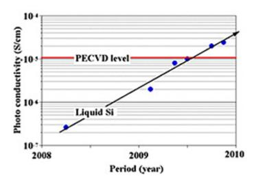
The problem of forming an uniform polysilane film was solved by carefully examining controlled parameters and optimizing the burning conditions of the polysilane film and reduced the density of the unattached hands to  $1 \times 10^{16}$ /cm<sup>3</sup>.
