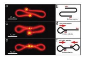
(A, C, E) Photoluminescence microscopy images of single-nanowire lasers in three configurations. (B, D, F) The thin arrows represent endface reflection with low reflectivity, while the thick arrows represent loop mirror reflection with high reflectivity. Image credit: Yao Xiao, et al. ©2011 American Chemical Society.
