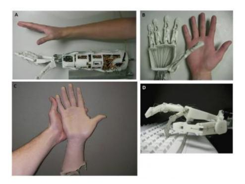
(A) and (B) show the DART hand in comparison to a human hand. (C) shows the silicone skin covering the mechanical components. (D) shows the DART hand typing the letter 'L' at a computer keyboard. Image credit: Thayer, et al. ©2011 IOP Publishing Ltd.
