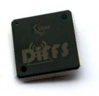
Caption: Imec's digital front-end for low-cost and low-power spectrum sensing.
