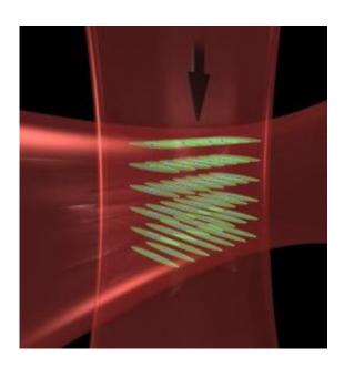
Intersecting laser beams create "optical tubes" to pack atoms close together, enhancing their interaction and the performance of JILA's strontium atomic clock. Credit: Baxley/JILA
