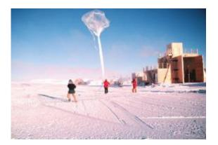
NOAA scientists launch an ozonesonde via balloon to measure of the vertical profile of the ozone layer. NOAA releases ozonesondes at eight sites worldwide, including the Amundsen-Scott South Pole Station. It also uses satellite and ground-based systems to continuously monitor stratospheric ozone.
