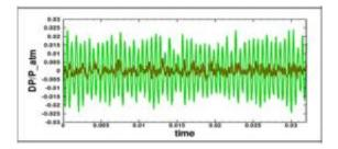
Reduction in pressure fluctuations (and hence noise) with mechanical chevrons (brown) in comparison to the baseline case without chevrons (green) at a representative location outside but near the jet.
