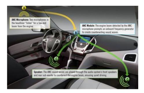
The technology that makes high-end noise-cancelling headphones coveted by frequent flyers and iPod audiophiles is helping GMC Terrain owners save gas. Active noise cancellation does double duty on Terrain. The technology enables the crossover to deliver a segment-leading EPArated 32 mpg in highway driving while ensconcing the driver in one of the quietest interiors in its segment. On the highway, Terrain easily tops the 28-mpg rating of Honda CR-V, Toyota RAV4 and Ford Escape.
