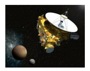
An artist's rendering of the New Horizons spacecraft as it approaches Pluto. The prominent 2.1-meter dish antenna is used to communicate with Earth from up to 7.5 billion kilometers away. Credit: JHUAPL/SwRI
