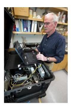
Scott Gallager works on the swimming behavioral spectrophotometer to analyze the safety of a water sample. Credit: Tom Kleindinst Copyright Woods Hole Oceanographic Institution (WHOI)
