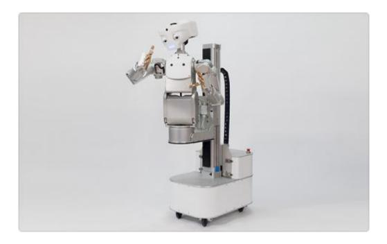
The choice of using modified Microsoft Kinect <u>sensors</u> allows the <u>robot</u> to see the world in some semblance of 3D, which is important if the <u>robot</u> wants to be able to act in the real world, which is the goal of these bots, human-like action.
