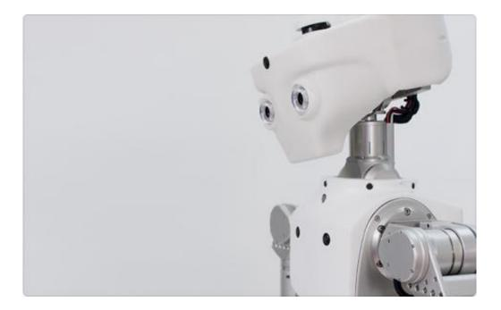
(PhysOrg.com) -- San Francisco-based company Meka has introduced the Meka Robotics' M1. The Meka Robotics' M1 is a mobile robot that features a pair of dextrous arms with what is known as compliant forcecontrol (a set of sensors that measure how much force is being used for each task, in order to keep the robot from breaking items or hurting humans) and some modified Microsoft Kinect sensors.
