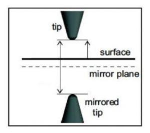
The sharp, magnetized tip of the probe used in this study induces an answering field in the superconductor in a phenomenon called the Meissner Effect. The strength of the response at each point gave SIMES researchers new information about the superconducting state of the pnictide. (Image courtesy Lan Luan)
